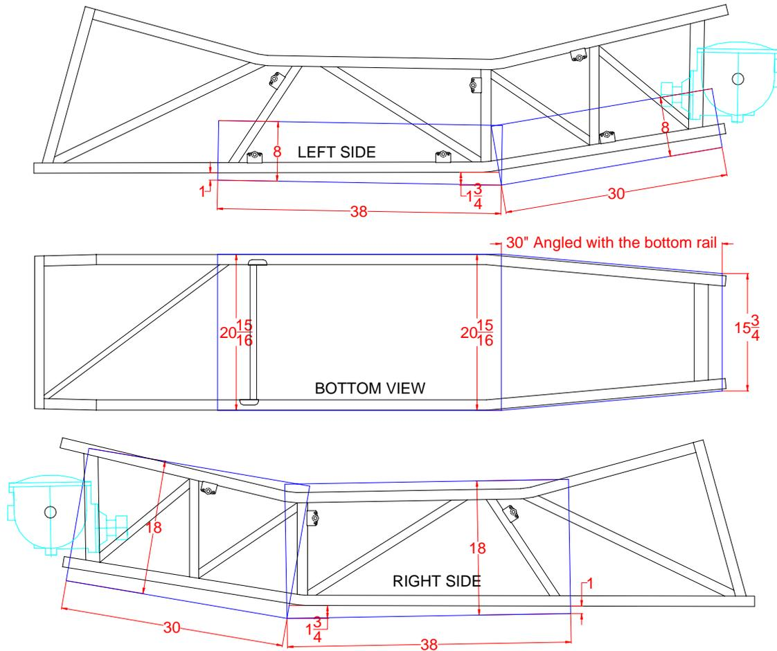
The dimensions above represent a standard Belly Pan Kit. If these do not work for your application, these sizes can be altered. The left side of the belly pan is left short so that the pan may be removed from the chassis over the Pro-jack tabs. An additional left side panel is included with the kit to cover the left side of the chassis to the top rail. The width and length of the pans are the critical dimensions required to bend a custom size belly pan.
