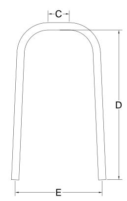
"C" is the length of straight required. This dimension will be the amount of flat needed, **NOT** the bend to bend dimension.
